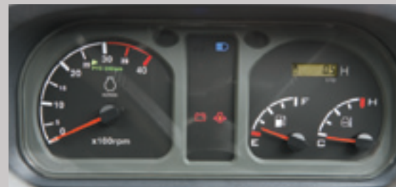
LED Instrument Panel Easy-to-read instrument panel includes gauges for engine RPM, engine temperature, fuel level, as well as a digital hour meter and PTO on/off indication light
